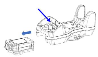
3. Replace the module by inserting it into the cradle, lock the lever and screw the module to the cradle.
